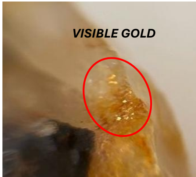
Photo 3: Visible gold observed in drill hole NMWBAC25-897: 41-42 metres. Returned a composite gold grade of 4 metres @ 2.8 g/t Au (within 8 metres @ 1.47 g/t Au) from 40 metres
