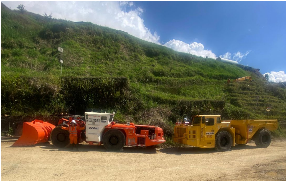
Photo 8: Mobile Mining Equipment commissioned on site, June 2025 (Load Haul Dump vehicle and underground truck)
