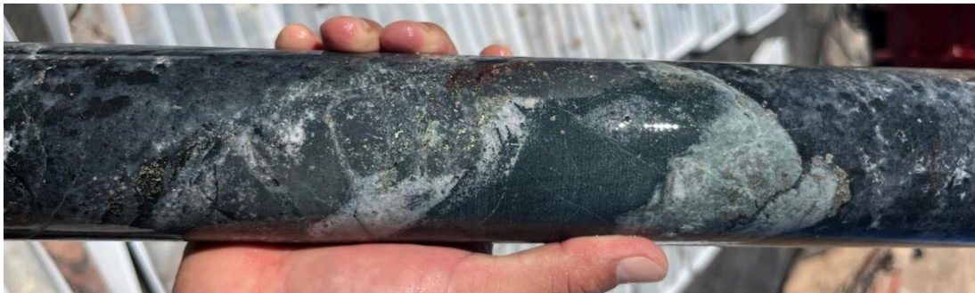
Figure 4: CAP-001-2025 drill core from 184.20 to 184.75 metres displaying tourmaline/specularite breccia with chalcopyrite mineralisation hosted in diorite intrusive. Visually estimated grade 0.5% Cu 1 . Assays are due for release in August 2025.
