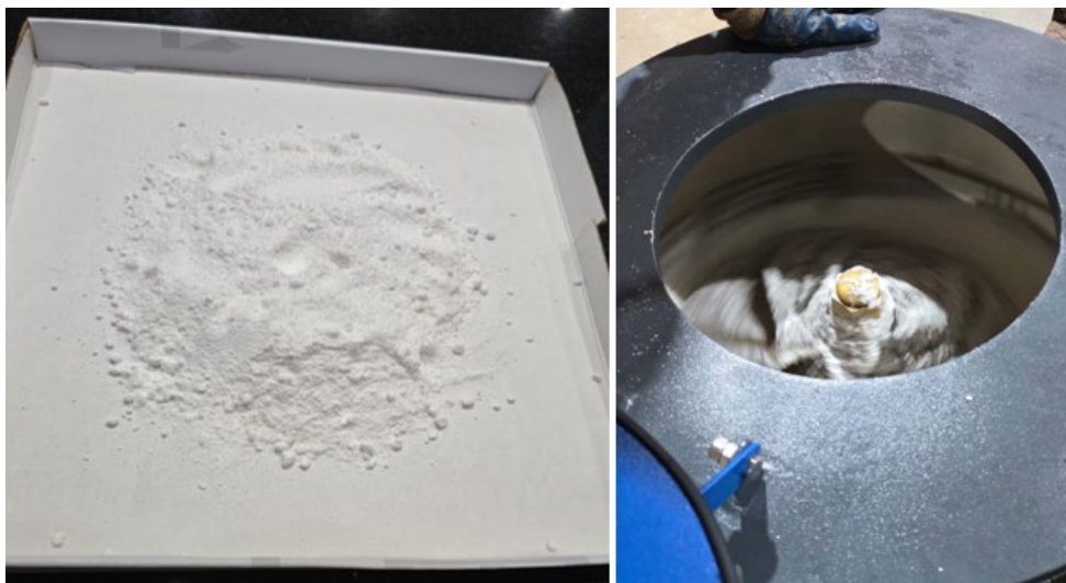
Figure 4: 98.9% Lithium Carbonate (left) and processing in the plant’s centrifuge (right)
