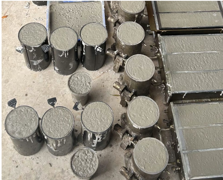
Figure 6: Concrete sample preparation
