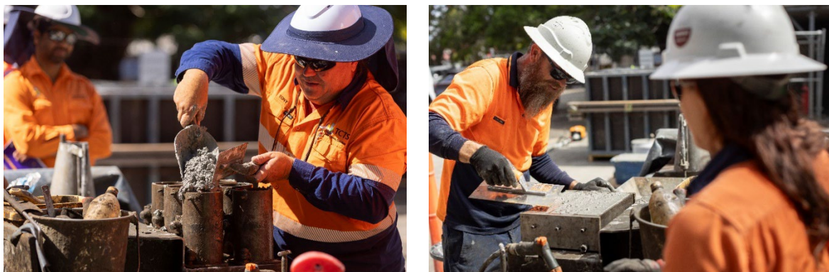
Figure 3: Concrete samples collected for independent testing
