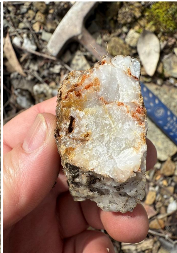
Figure 8 – Gold mineralisation within ferruginous quartz vein yielding 25.2 g/t Au from sample 3001649
