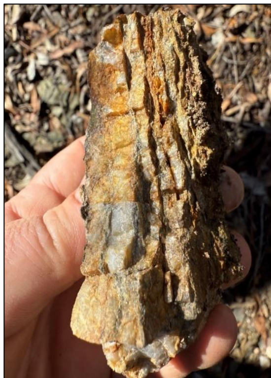
Figure 4 – Gold mineralisation within ferruginous quartz vein yielding 51.4 g/t Au from sample 3001533
