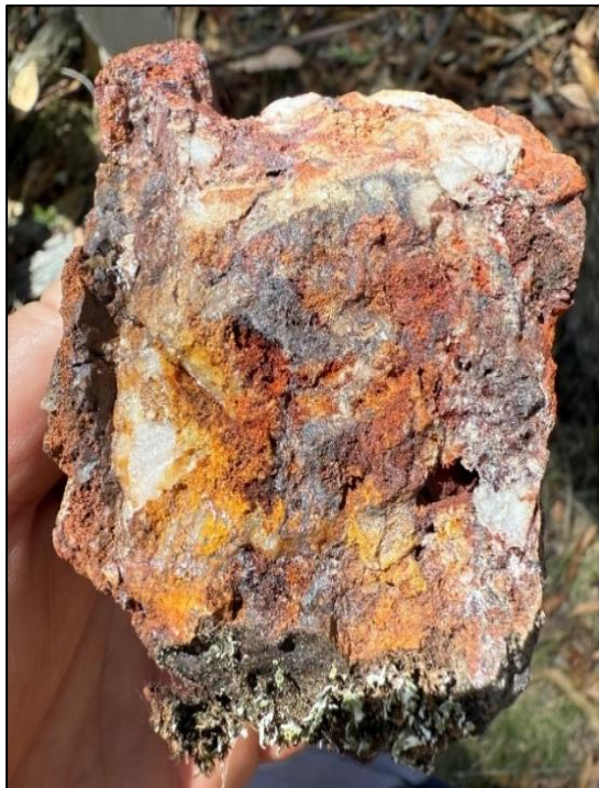
Figure 3 – Gold mineralisation within iron rich quartz yielding 216 g/t Au from sample 3001522
