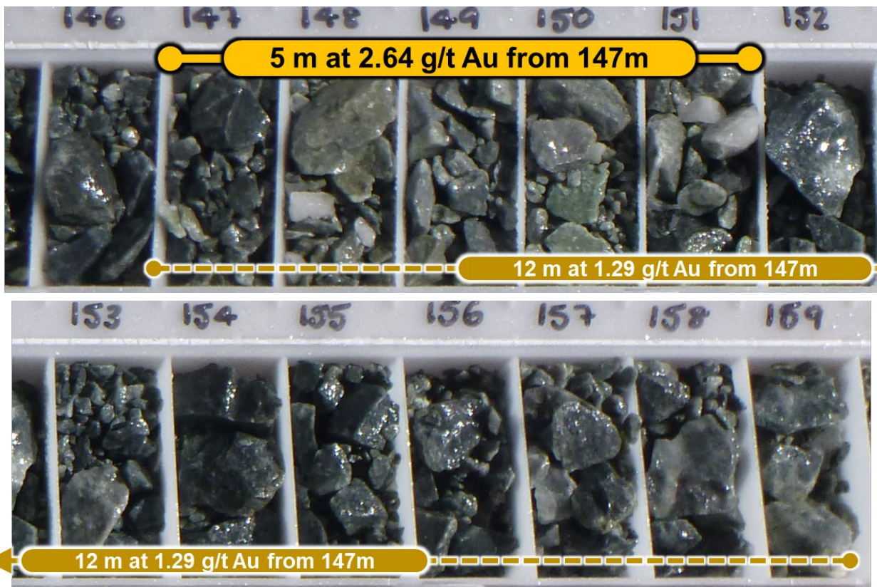
Figure 2 – RC Drill chips from hole KGRC25014 showing the mineralised interval 147-152m (5m at 2.64g/t Au), within a broader zone of sub-grade anomalism from 147m (12m at 1.29 g/t Au). Green- to buff-coloured sericite-silica-carbonate-chlorite alteration (locally with pyrite) is directly associated with quartz vein fragments (white), depicting useful visual indicators for gold mineralisation at Lighthorse.
