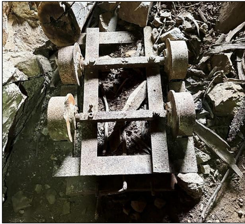
Photo 5. Magwood mine ore cart. Primitive historical mining methods resulted in only the highest-grade antimony mineralisation being mined and hand sorted
