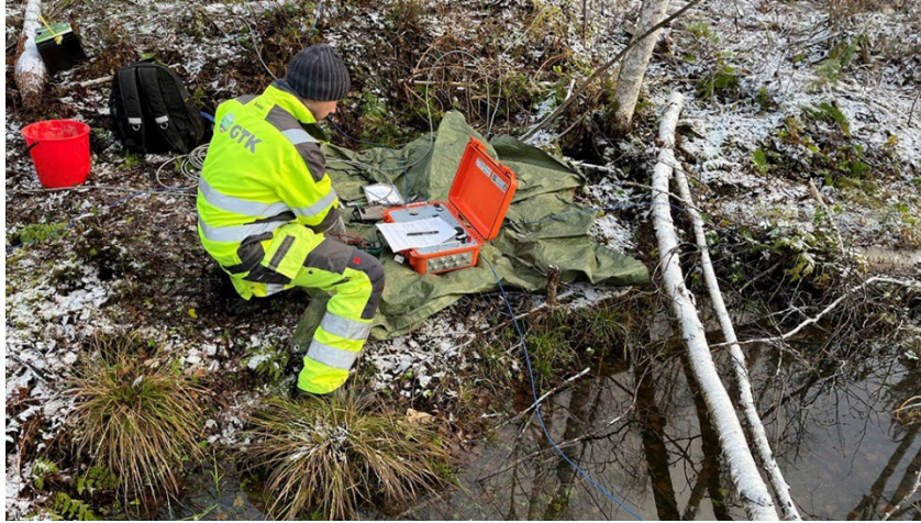
Figure 10: Installation of magnetotelluric measuring equipment
