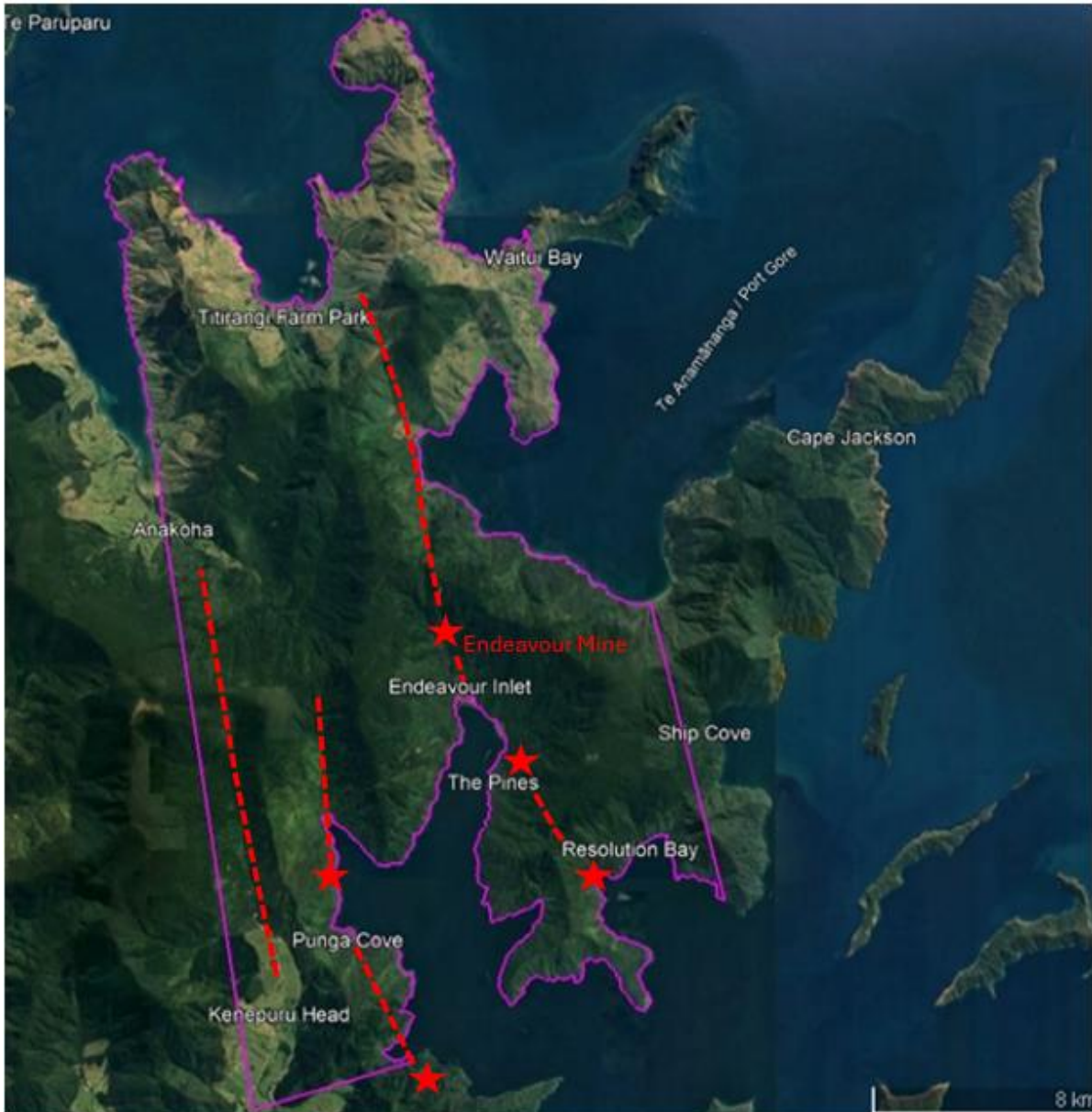
Figure 24: Exploration permit (purple line), Potential shear zones (red dotted lines) and outcropping antimony mineralisation (red stars).
