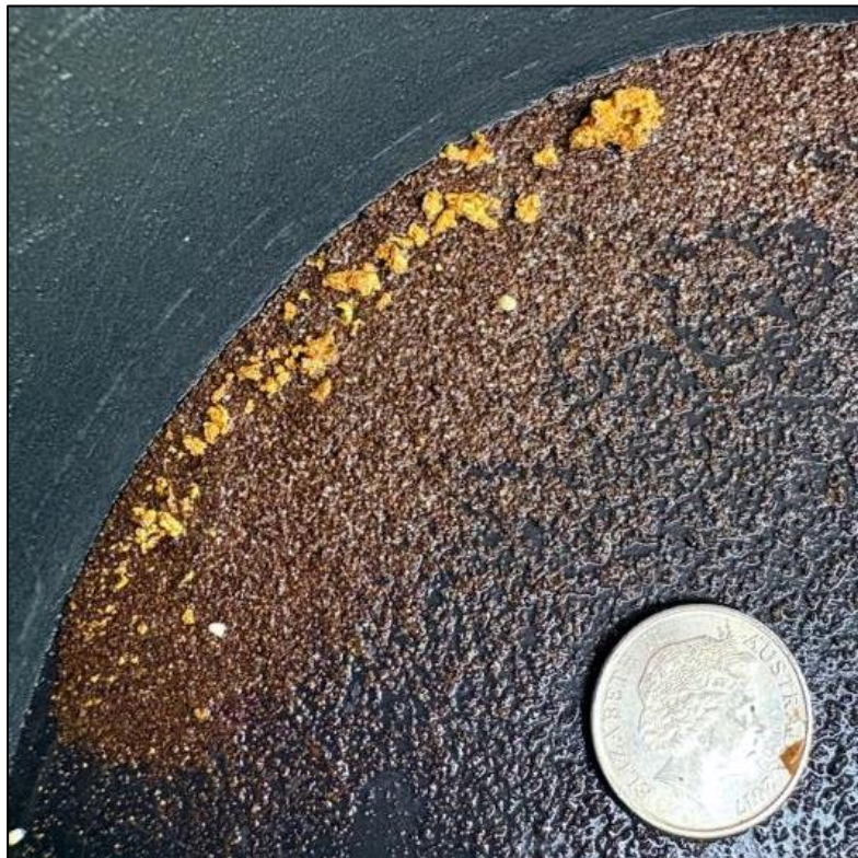
Figure 16: Visible Gold recovered from panning the bulk 1m sample for the interval 37-38m in drill hole INRC25073, which reported 1m at 356g/t Au. Coin for scale is approximately 20mm in diameter.
