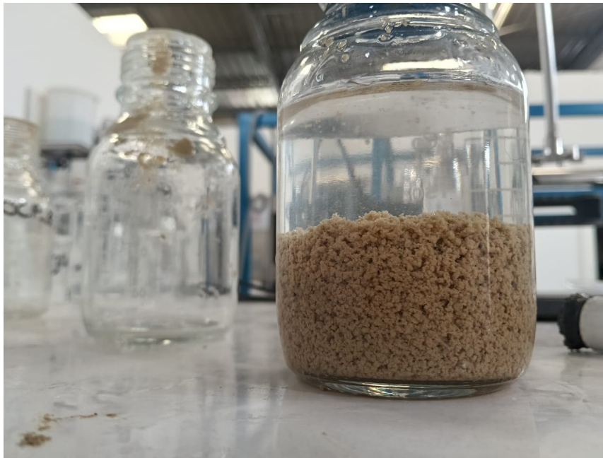
Bench-scale testwork showing rapid separation of solids and water with ATA®
