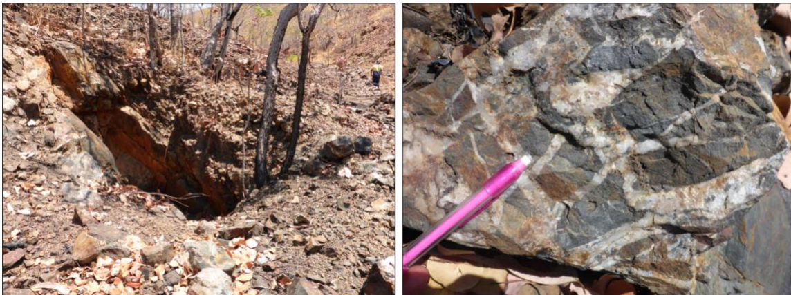
Figure 8: Grants historic working and rock chip sample (LW0014) of mullock grading 275 g/t Au.
