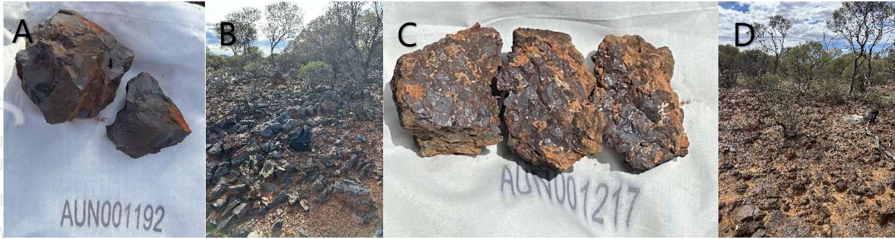
Figure 12. (A) Hematite enriched BID (Sample AUN001192 – 65.17% Fe), (B) outcropping hematite enriched BID, (C) hematite enriched capping / pisolite (Sample AUN001217 – 59.62% Fe), (D) outcropping cemented hematite pisolite potentially representing immature paleochannel iron deposits or capping. Results are presented in Annexure E.
