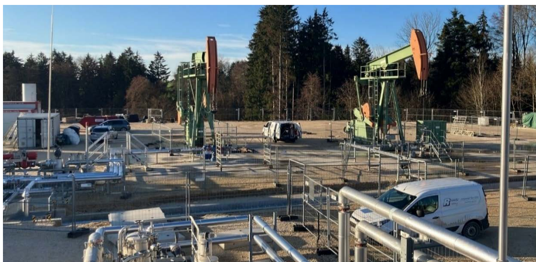
Photograph showing the Anshof-3 well (left side, photo) and the Anshof-2A well (right side, photo) producing into the Anshof PPF
