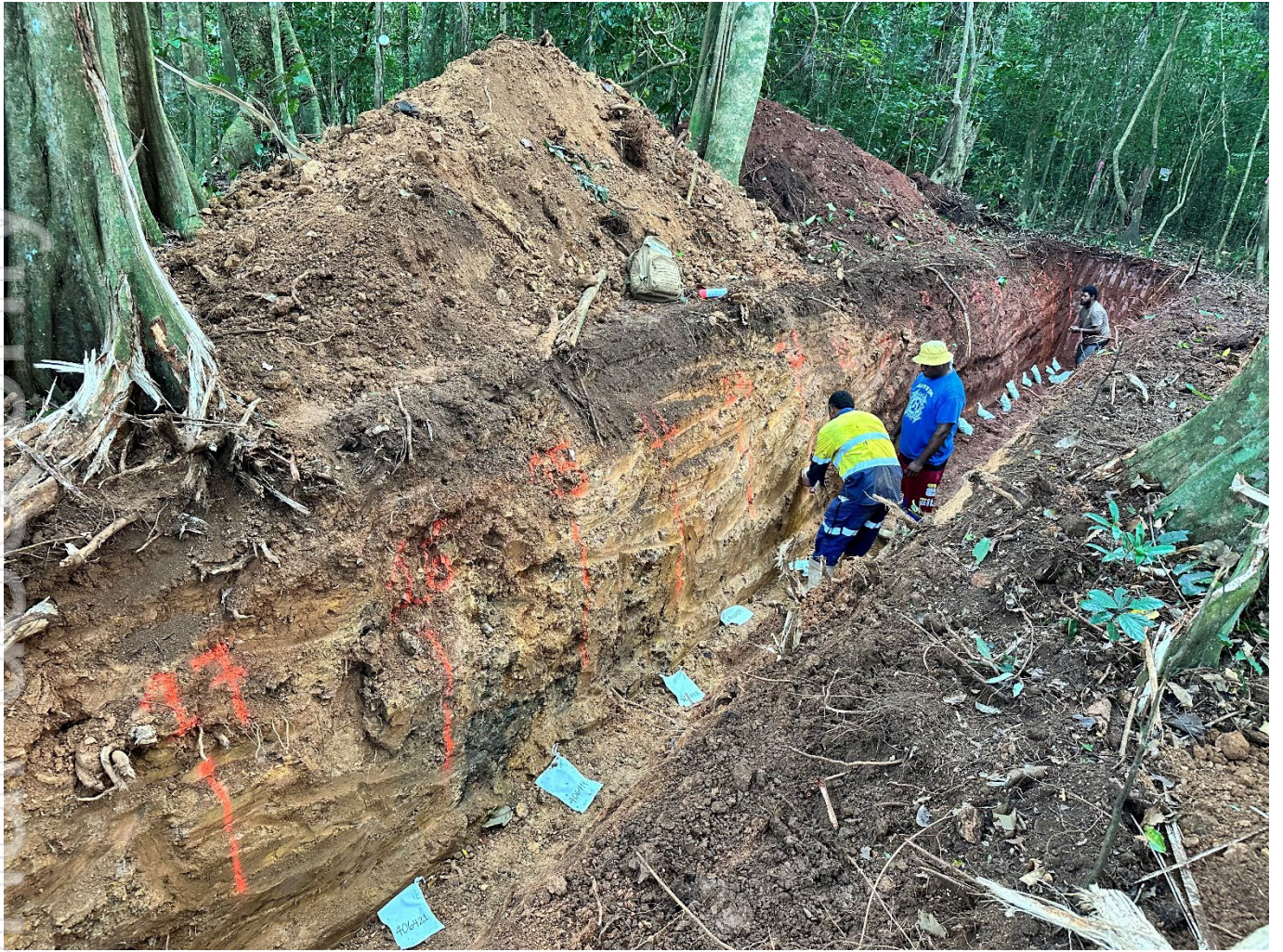
Figure 4 – Channel sampling one of several costeans across the mineralised strike during the June Quarter.
