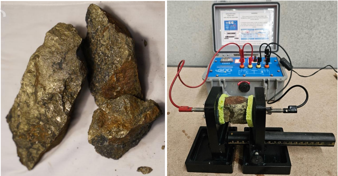
Figure 7: Prince Of Wales prospect sample RK008302 10.15% Cu and 65.8g/t Ag 12 , being tested for Induced Polarisation, chargeability, galvanic resistivity and inductive conductivity
