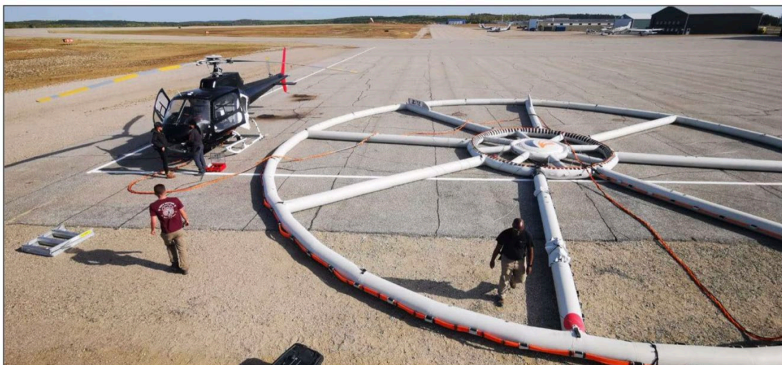
Figure 6: Configuration of Xcite™ TDEM survey system.
