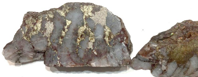
Figure 3b: Photograph: approximately 10cm length of broken core displaying the Cu-Mo hosting sulphide minerals within a quartz vein. Specimen from 160.16m drill depth in hole D28-DDH4
