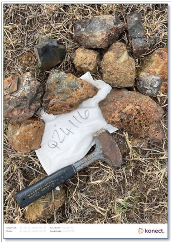
Photo 3: Breccia of altered siltstone/sandstone in a fragmental but weakly silicified groundmass. Some occurrences show limonite or goethite filled boxwork that may have been after a sulphide
