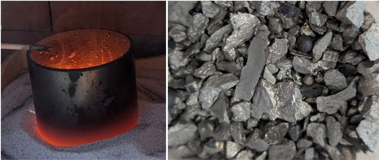
Figure 6: Conversion vessel with ferroniobium cooling following the test (left) and ferroniobium alloy (right)
