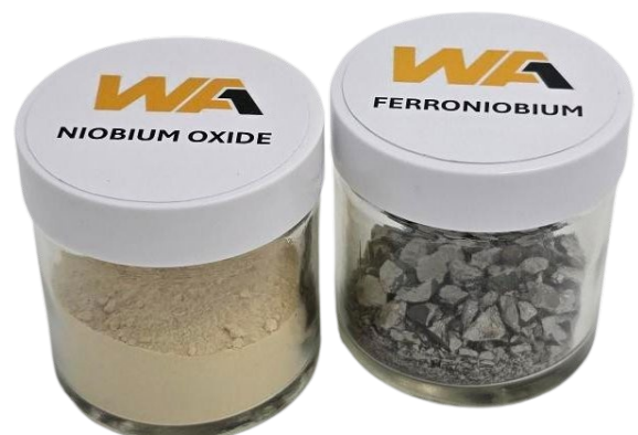
Figure 1: Niobium oxide and ferroniobium from recent testwork
