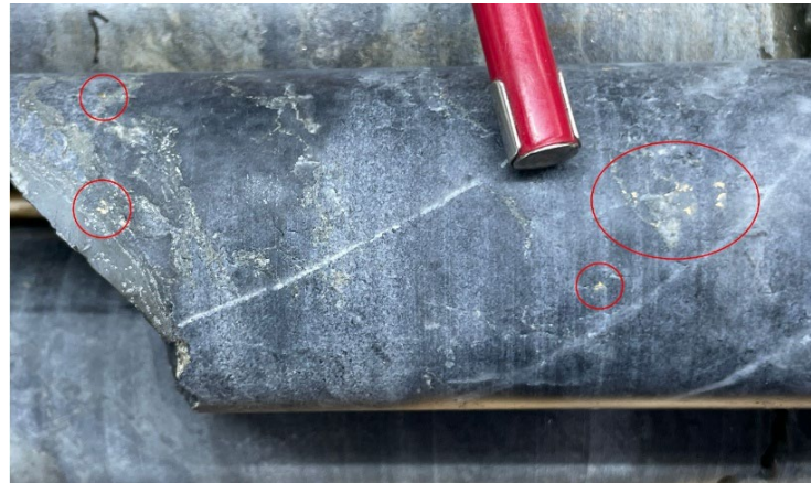
Photo 2 (RHS): Visible gold grains in 20cm smoky quartz vein hosted in sulphide, chlorite-carbonate altered wacke, 187.8-187.9m, BO-25-27. Core diameter is 4.76 cm. Assay results 187.5 – 187.85m 42.3 g/t Au (see Table 1).
