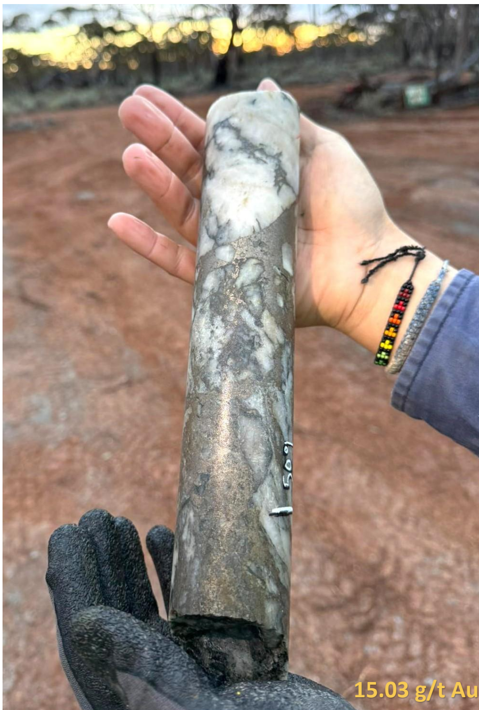
Figure 4 Core at 508.82m to 509.2m (grading 15.03 g/t gold) displaying semi-massive sulphides as pyrrhotite chalcopyrite arsenopyrite breccia with quartz carbonate veining and chlorite alteration. Type of veining and alteration often associated with orogenic gold systems, near structural feeders.
