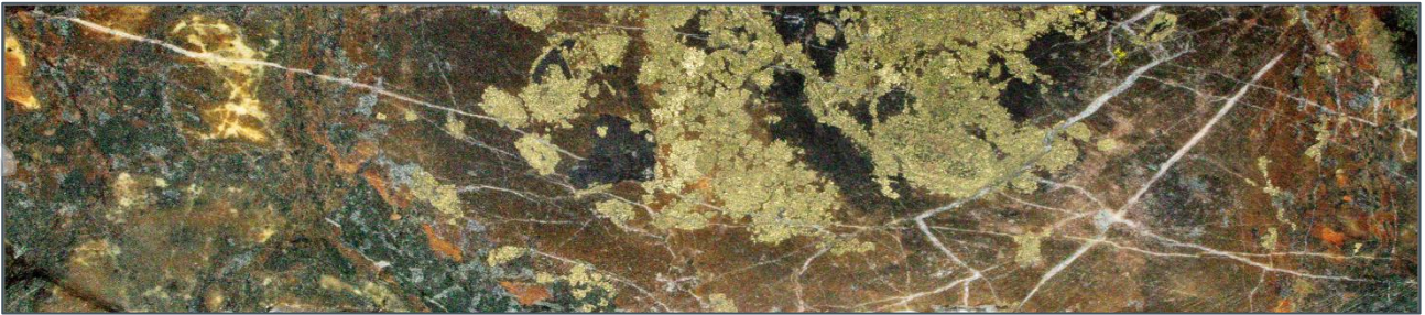
SPRCD062 - 464.9m – Patchy and veinlet associated pyrite ± chalcopyrite with pervasive k-feldspar alteration, 1.0g/t Au
