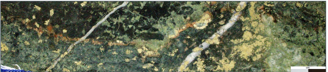
SPRCD062 - 596.3m - Patchy and veinlet associated pyrite ± chalcopyrite with pervasive chlorite alteration, 2.56g/t Au
