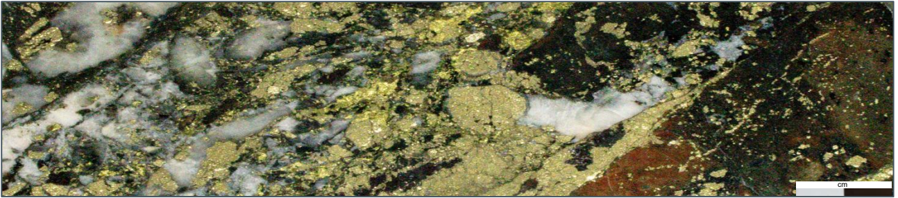
SPRCD062 - 592.6m – Patchy and veinlet associated quartz + pyrite ± chalcopyrite with pervasive k-feldspar + chlorite alteration, 4.45g/t Au
