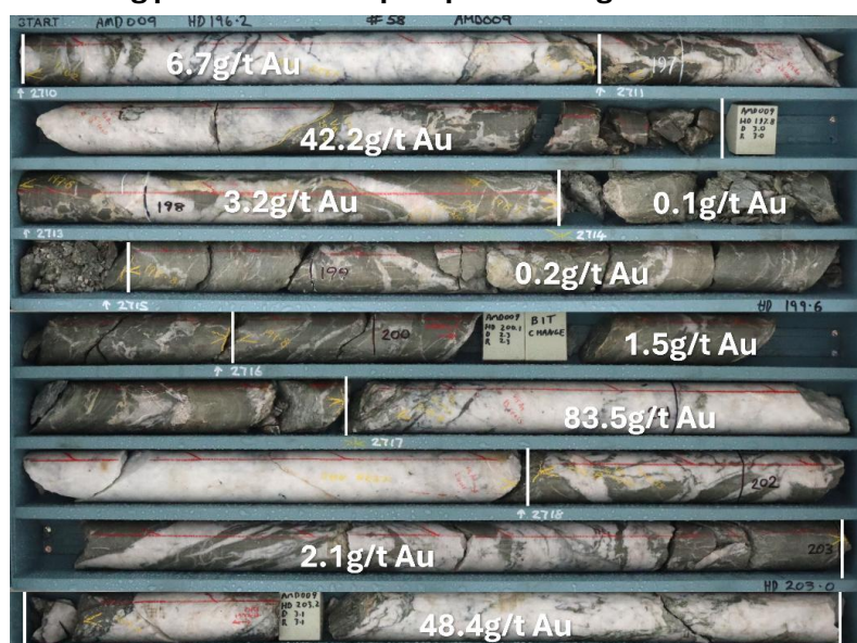
Figure 1. Composite photograph of core from AMD009 highlighting individual down hole gold grades from 196.2m. This zone graded 9.4 metres at 20.2g/t Au .
