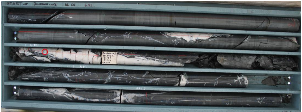
Figure 6 Laminated quartz vein with trace of visible gold at red circle. Interpreted to be T734
