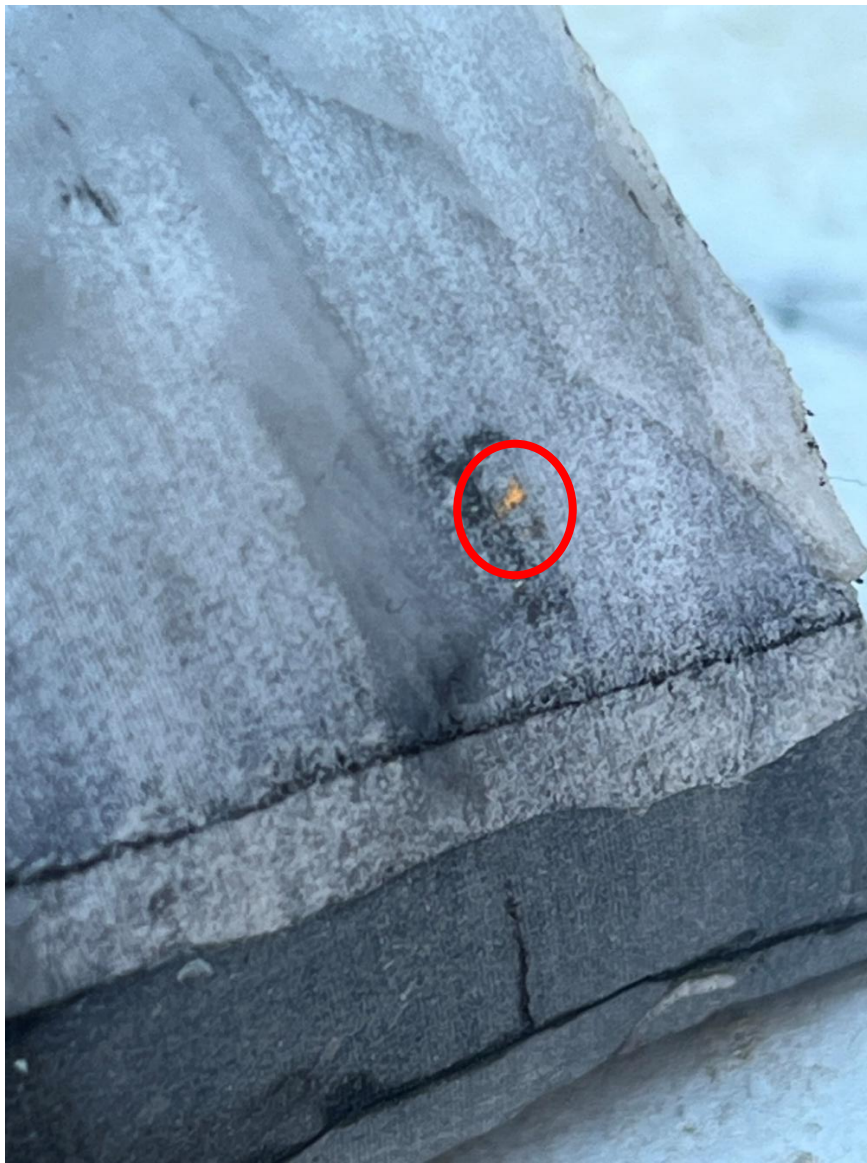
Figure 7 Close up of visible gold (~1mm across) at 680m within the red circle in the NQ core
