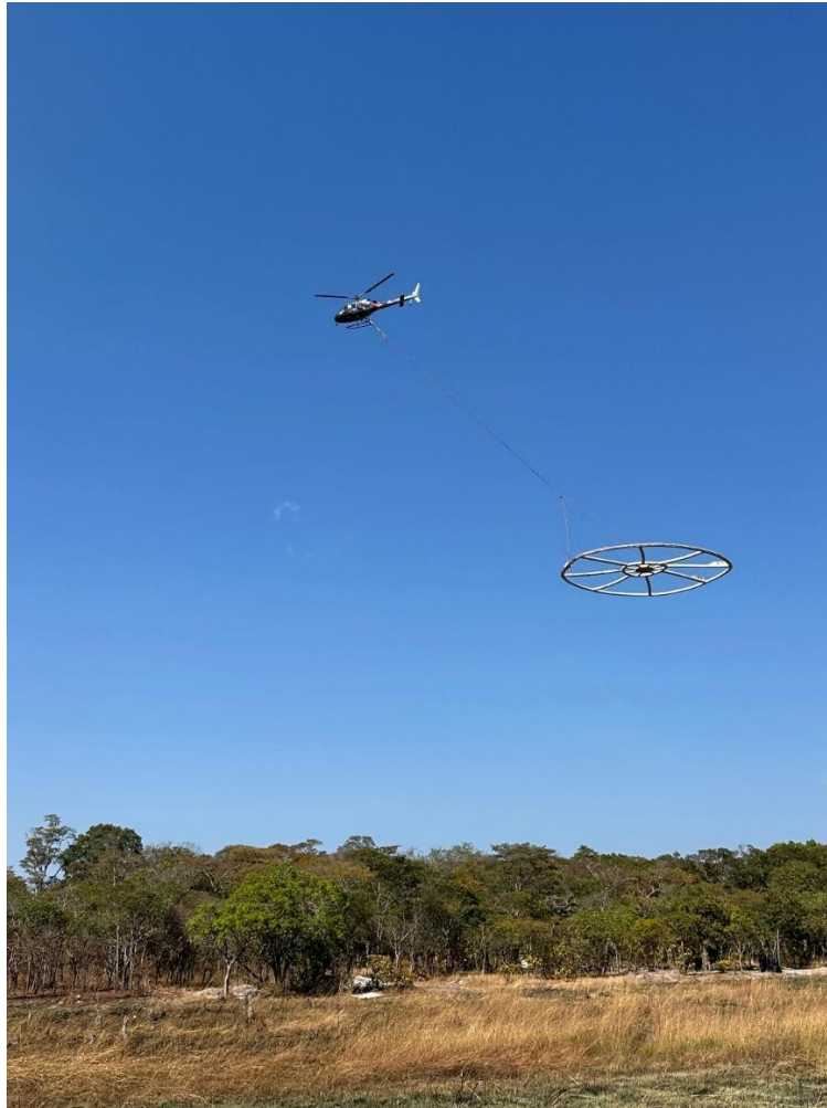
Figure 5. Airborne Electromagnetic (EM) Geophysical Survey underway at Mumbeshi Project
