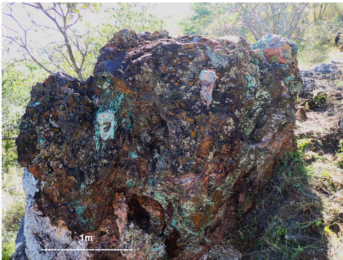
Image 1: Area 6, Gossan 1 Outcrop. Malachite (copper-carbonate) and iron oxide (after sulphides) in brecciated dolomite. Five rockchip samples, A6SM5, 6, 7, 8, 9, averaged 18.6% Cu, 18.4% Zn, 1.3% Pb, 427g/t Ag, 20 g/t Ge – see Table 1 & Appendix 1
