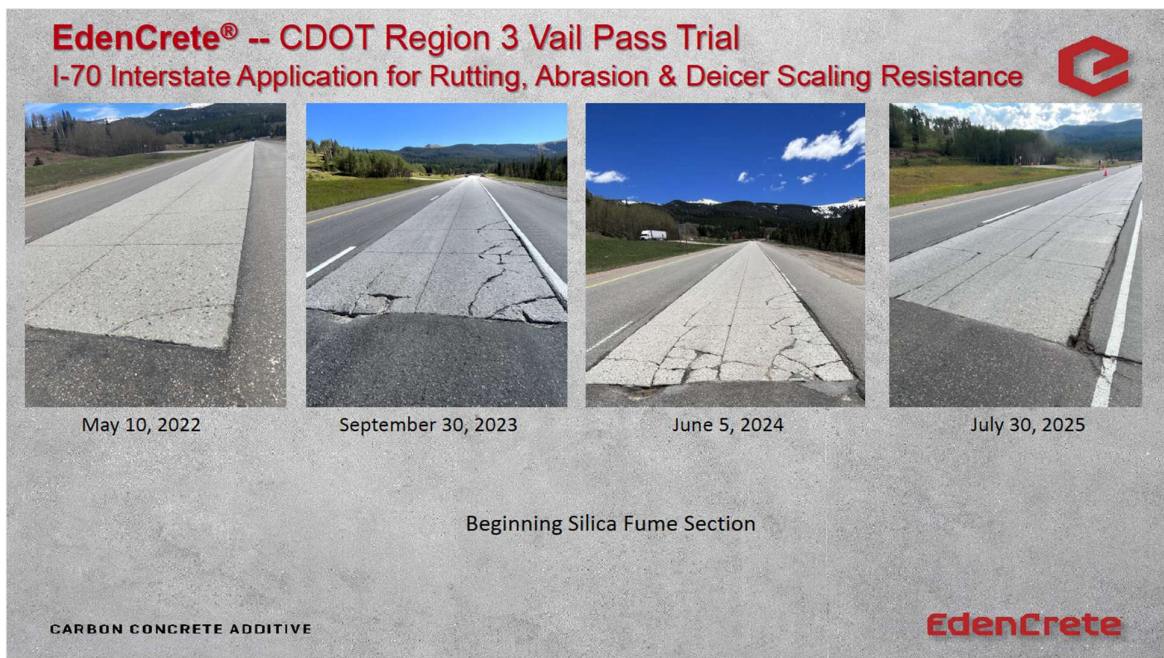
Figure 3. Silica Fume concrete – Beginning Section ( 2 panels at the start replaced with bitumen to remove safety hazard).
