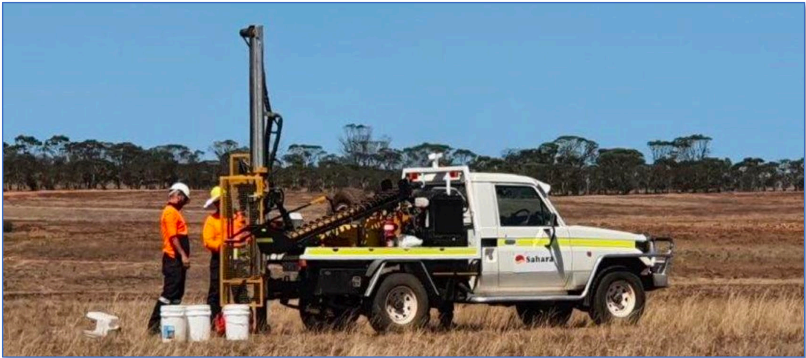
Fig 2: Sahara Mining Services auger drilling rig.
