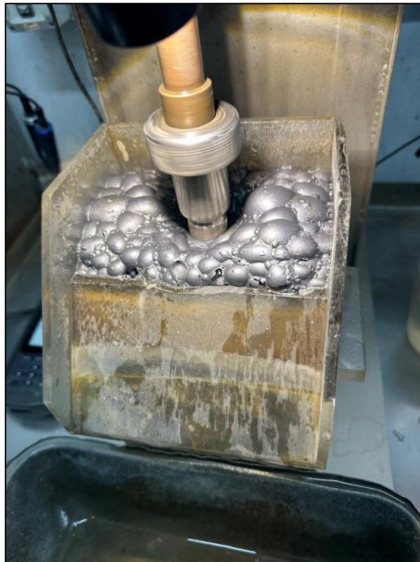
Figure 2: Photo of flotation cells with Achilles metal-bearing sulphides being floated
