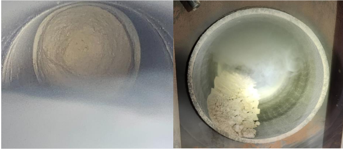
Figure 8: Adhesion Inside Rotary Kiln During Sulfuric Acid Roasting of Hammer Mill Crushed Samples(left) and Cutter Mill Crushed Samples After Sulfuric Acid Roasting
