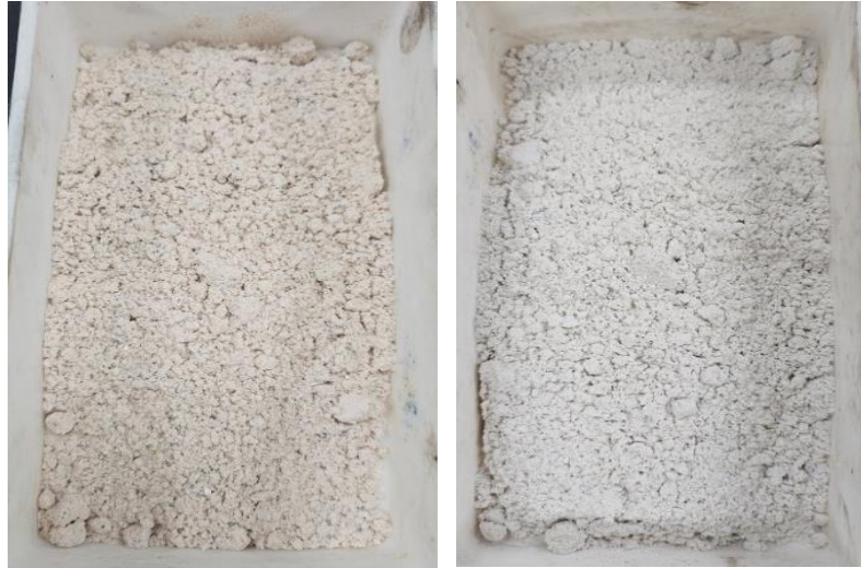
Figure 2: Before (left) and After (right) Sulfuric Acid Roasting After Mixing with Sulfuric Acid
