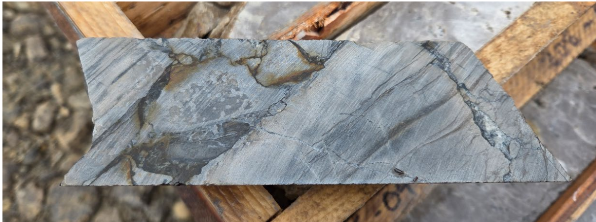
Figure 1: Dense crackle breccia with visual chalcocite (copper sulphide) and fine pyrite from drill hole ST25-04 (210.6-210.75m downhole). Assays for this interval are pending.
