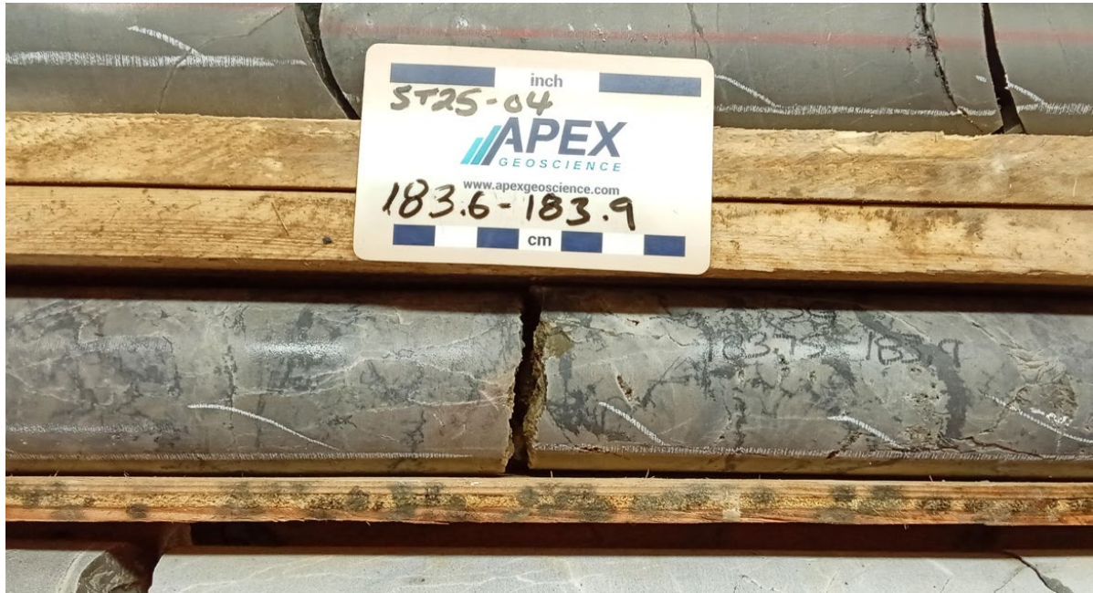
Figure 2: Dense breccia and fracture fill visual pyrite and chalcocite (copper sulphide) from ST25-04 (183.6-183.9m downhole). Assays for this interval are pending.
