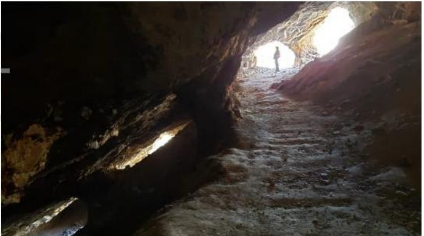
Figure 3. Near surface open stope from historic mining on the Rosario Vein at Guadalupe y Calvo.
