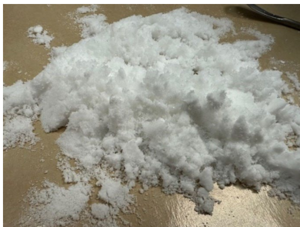
Figure 10.6: Boric acid crystals after re-crystallization and dewatering process
