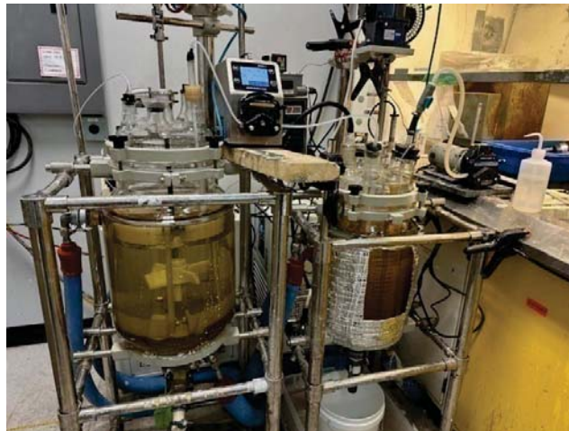
Figure 10.2: Boric acid continuous crystallization set-up including an agitated feed tank
