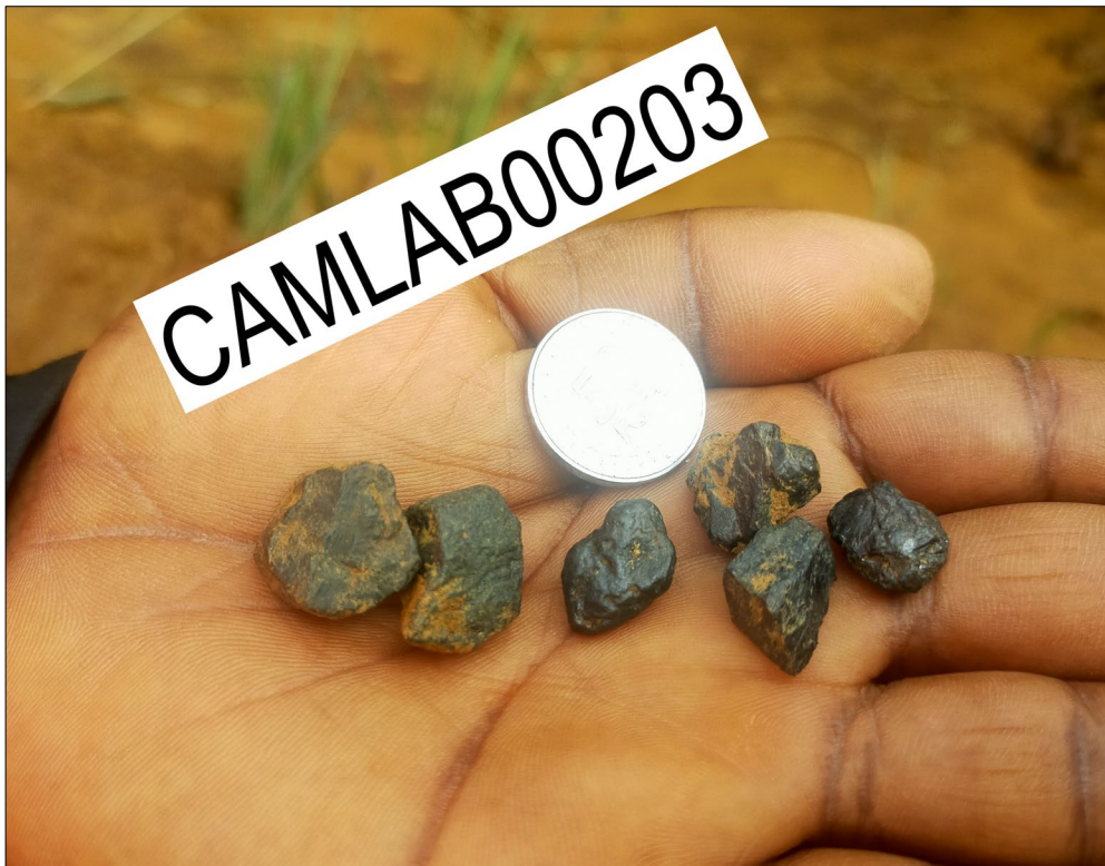
Figure 4: The rutile nugget displays a massive texture, with some grains exhibiting elongation. The rutile displays a sub-metallic lustre with dark grey to black colour with secondary Fe-oxides and sub-rounded crystal suggesting limited lateral transport. XRF results in Table 2 and Appendix II
