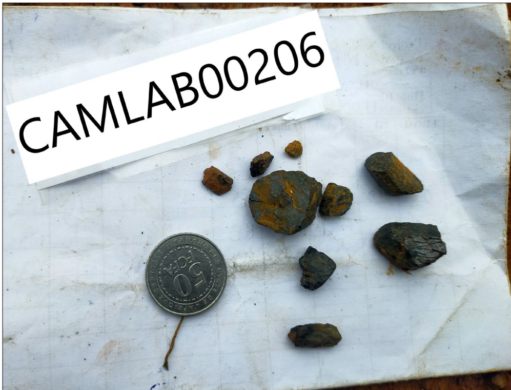
Figure 2: The rutile nuggets display a massive texture, with some grains exhibiting elongation. The rutile displays a sub-metallic lustre with dark grey to black colour with minor secondary Fe-oxide coating and sub-rounded crystal suggesting limited lateral transport. XRF results in Table 2 and Appendix II.
