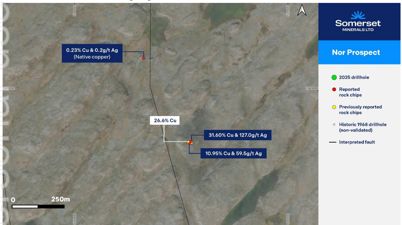
Figure 5: High-grade copper mineralisation at the Nor Prospect, including results up to 31.60% Cu & 127.0g/t Ag from surface rock chip sampling.
