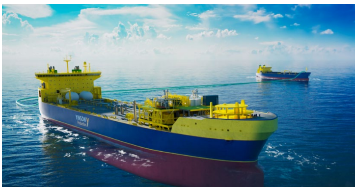
Illustration of a FSIU in the foreground, receiving cargo from a LCO2 carrier in the background (Source: Yinson Production AS)
