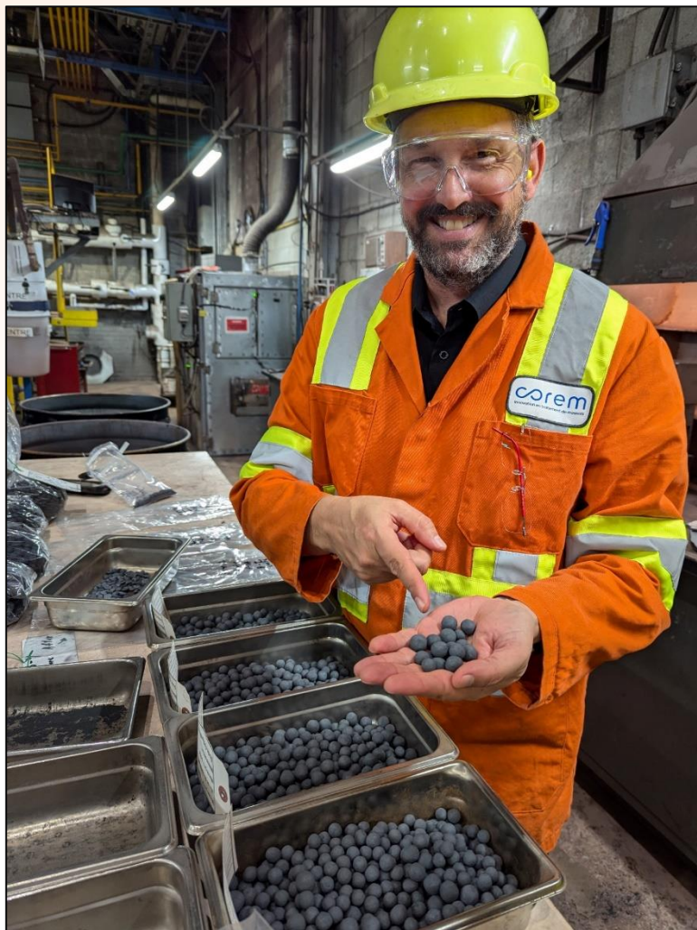
Figure 60: Iron Bear DR pellets produced at COREM
