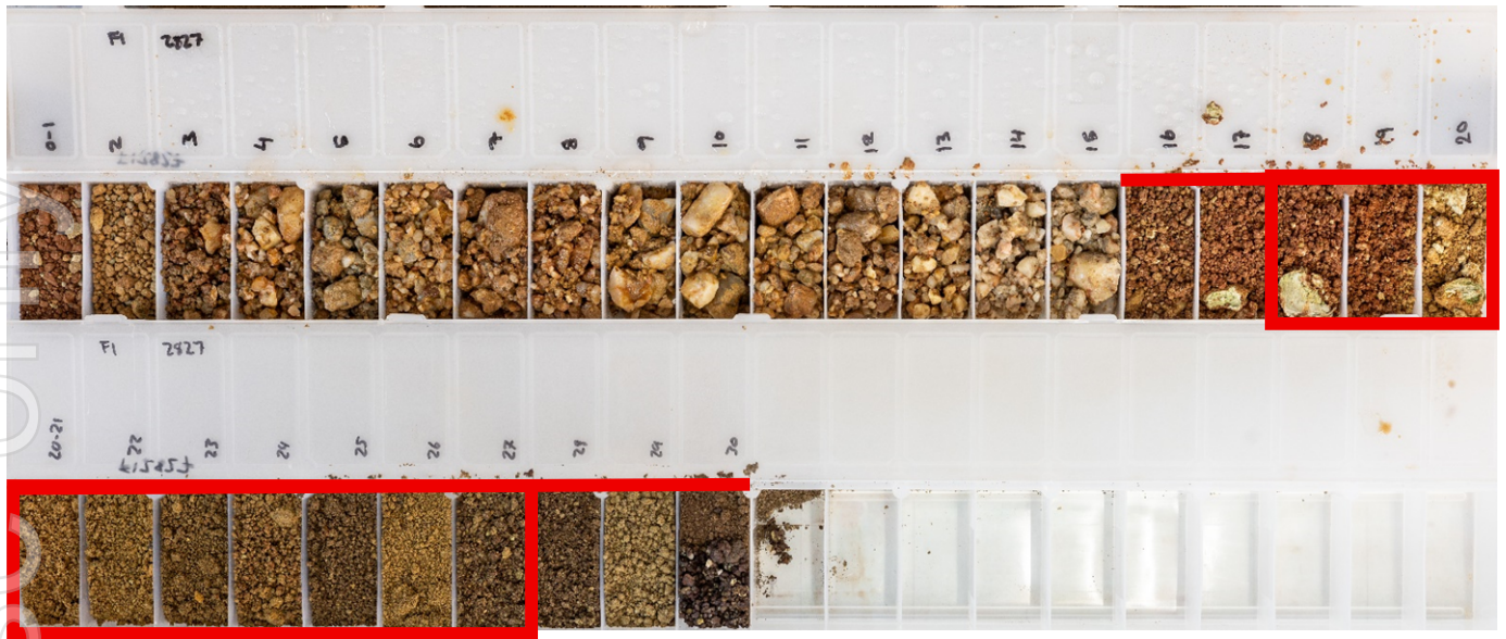
Figure 2: FI2827 chip tray photo with scandium interval highlighted - 15m @ 280 ppm Sc (429ppm Sc Oxide) from 15m including 10m @ 321ppm Sc (492ppm Sc Oxide). Each compartment in chip tray represents a 1 – metre downhole interval.
