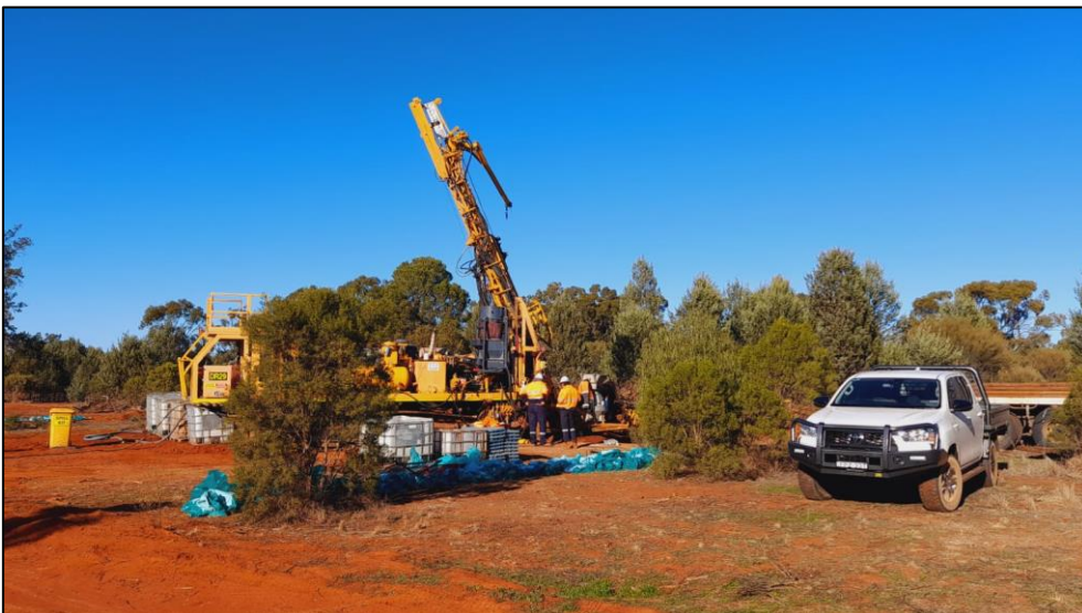
Figure 3: Diamond drill rig now set up at Achilles to test depth extensions to mineralisation. Diamond drilling uses a diamond encrusted tungsten drill bit to produce a core of rock.
