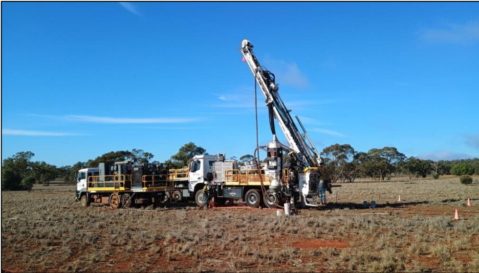
Figure 2: RC drill rig drilling the southern holes at Priority Target 1, photo looking south. This is an air driven technique that smashes rock with a hammer, producing 30-40kg rock dust in a sample bag per metre.
