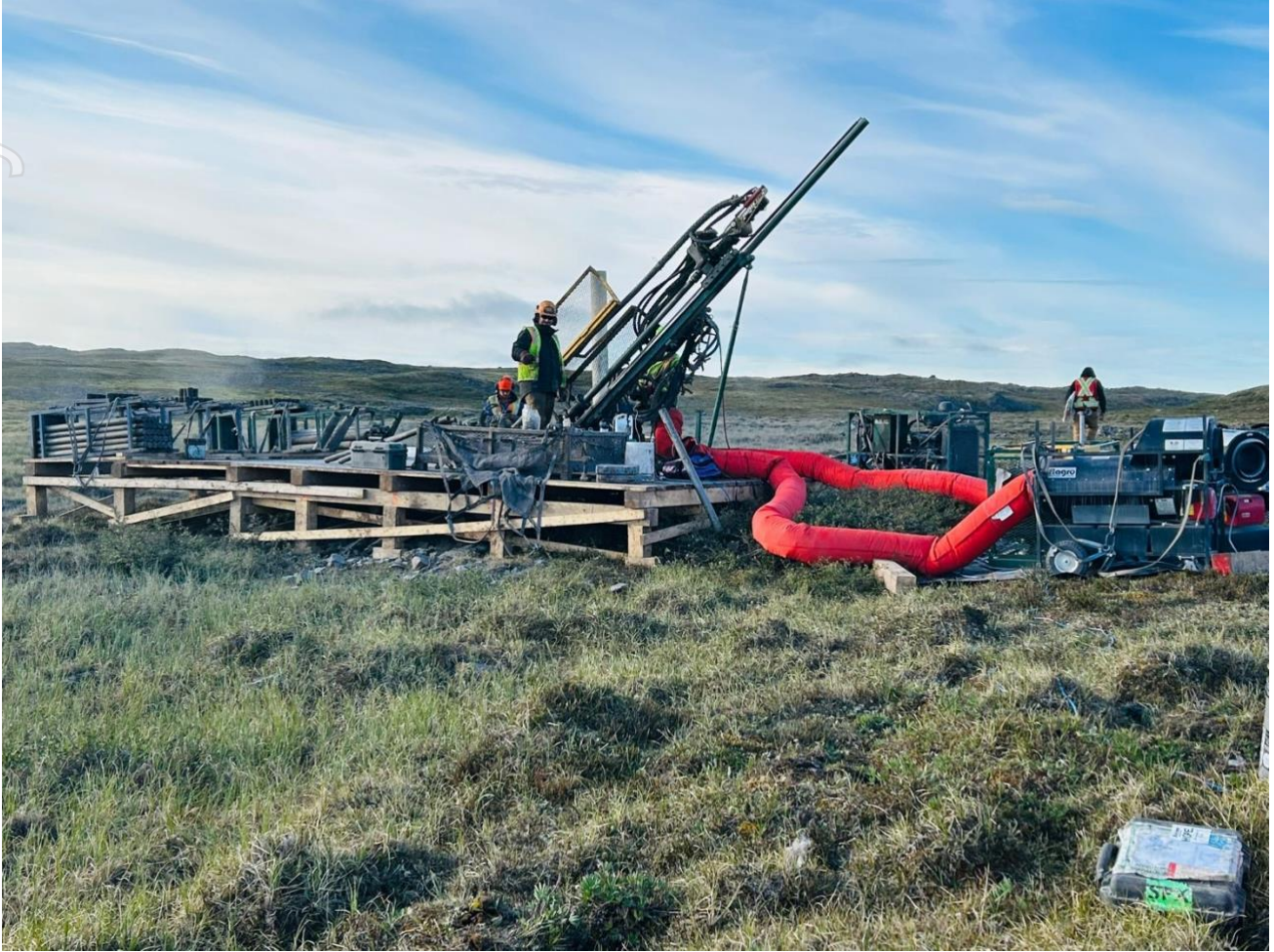
Figure 2 - Reverse circulation drilling underway at DAN25019.
