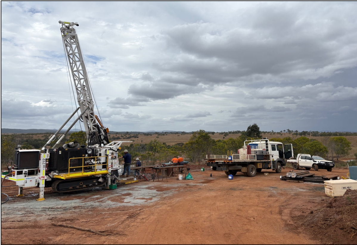
Figure 2: Diamond rig drilling first diamond tail at the Sulphide City deposit.
