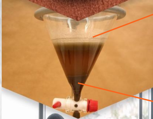
Photo 5. Laboratory HM separation via a heavy liquid
