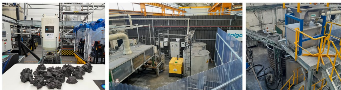
Fig 3: Recycled graphite anode concentrate feedstock (L) and Talnode®-R production pilot plant (C & R)
