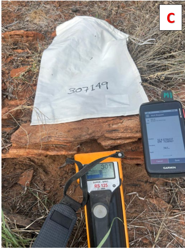
Figure 8: Rock chip sampling at the Treuer Range Project. Plate A: Rock chip sample collection during the inaugural Treuer Range fieldwork. Plate B: Rock chip sample 307104 using the RS-125 scintillometer to record Total Count Radiometric for Uranium-Potassium-Thorium ("K-U-Th") before sampling. Plate C: Rock chip sample 307149 using the RS-125 scintillometer to record Total Count Radiometric for Uranium-Potassium-Thorium ("K-U-Th") before sampling
