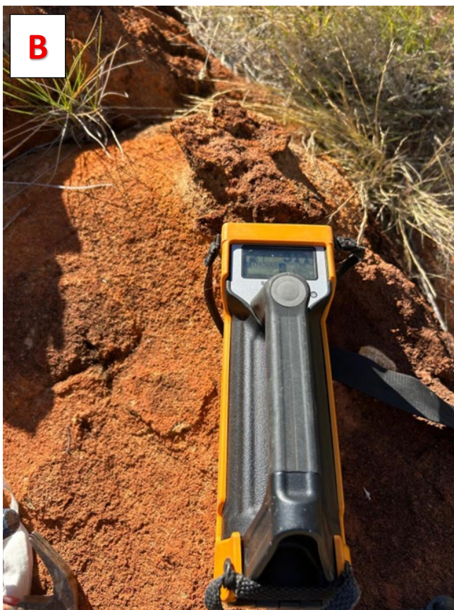
Figure 8: Rock chip sampling at the Treuer Range Project. Plate A: Rock chip sample collection during the inaugural Treuer Range fieldwork. Plate B: Rock chip sample 307104 using the RS-125 scintillometer to record Total Count Radiometric for Uranium-Potassium-Thorium ("K-U-Th") before sampling. Plate C: Rock chip sample 307149 using the RS-125 scintillometer to record Total Count Radiometric for Uranium-Potassium-Thorium ("K-U-Th") before sampling
