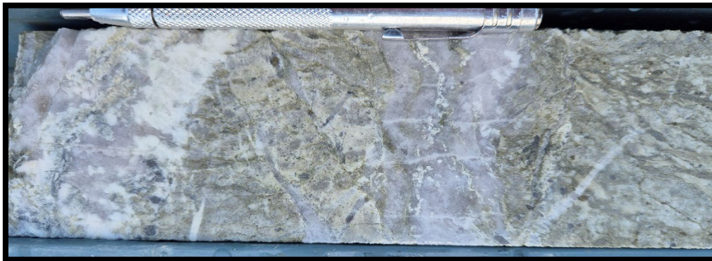
EPD017 – Sericite-carbonate altered dacite with sheeted quartz-albite veins and pyrite-arsenopyrite selvages from 6.1m interval grading 3.03 g/t Au from 120.9 m.
