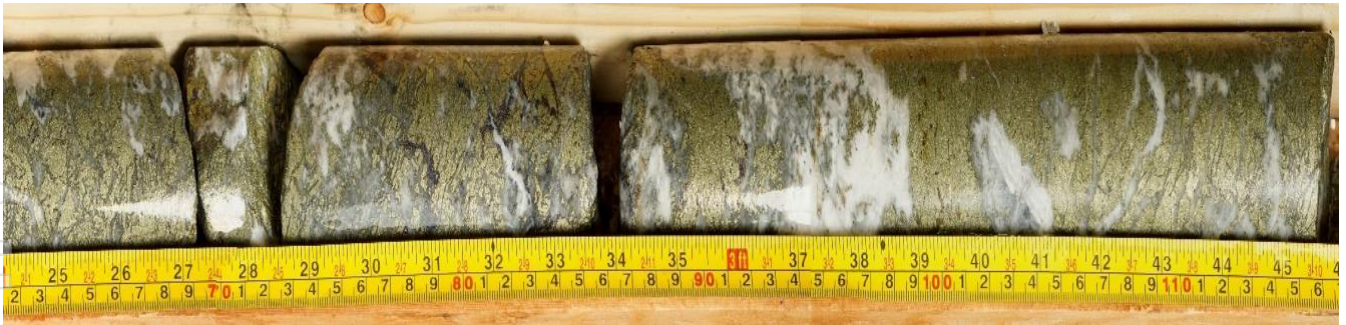
Figure 7 - Example of banded quartz-calcite epithermal veining with semi-massive chalcopyrite between 291.10 and 291.59m downhole in STK25001. Cautionary Statement: The Company cautions that, with respect to any visual mineralisation indicators, visual observations and estimates of mineral abundance and uncertain in nature and should not be taken as a substitute or proxy for appropriate laboratory analysis. Visual estimates also potentially provide no information regarding impurities or deleterious physical properties relevant to valuations. Assay results from the drilling and sampling programmes will be required to understand the grade and extent of mineralisation. Initial assay results are expected in the September quarter.
