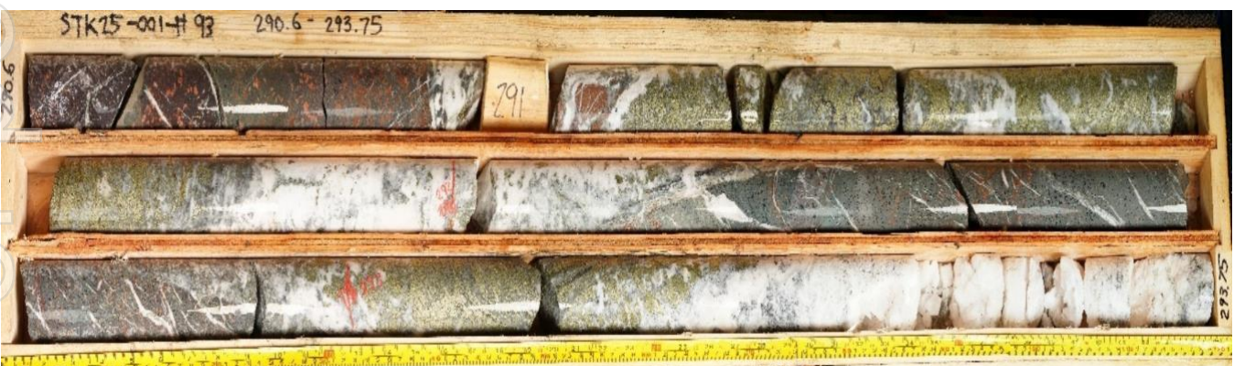
Figure 6 - Example of banded quartz-calcite epithermal veining with semi-massive chalcopyrite between 290.95 and 293.38m downhole in STK25001. Cautionary Statement: The Company cautions that, with respect to any visual mineralisation indicators, visual observations and estimates of mineral abundance and uncertain in nature and should not be taken as a substitute or proxy for appropriate laboratory analysis. Visual estimates also potentially provide no information regarding impurities or deleterious physical properties relevant to valuations. Assay results from the drilling and sampling programmes will be required to understand the grade and extent of mineralisation. Initial assay results are expected in the September quarter.
