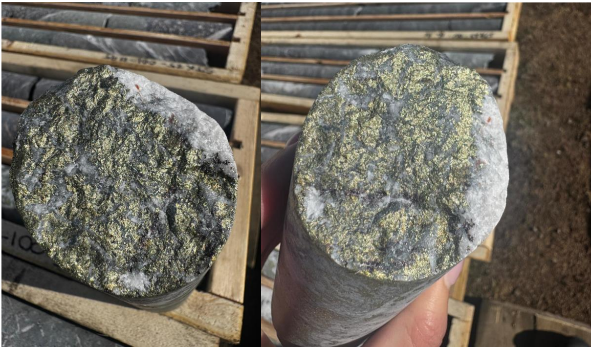
Figure 4 - Example of chalcopyrite-bornite-quartz-carbonate veining within the Husky Creek Formation of STK25001 at 291.4m. Core diameter is NQ2. Cautionary Statement: The Company cautions that, with respect to any visual mineralisation indicators, visual observations and estimates of mineral abundance and uncertain in nature and should not be taken as a substitute or proxy for appropriate laboratory analysis. Visual estimates also potentially provide no information regarding impurities or deleterious physical properties relevant to valuations. Assay results from the drilling and sampling programmes will be required to understand the grade and extent of mineralisation. Initial assay results are expected in the September quarter.
