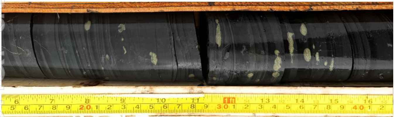
Figure 5 - Example of chalcopyrite replacement of inferred diagenetic pyrite nodules within reducing sediments of the lower Rae Group between 182.24 and 182.52m downhole in STK25001. Core diameter is NQ2. Cautionary Statement: The Company cautions that, with respect to any visual mineralisation indicators, visual observations and estimates of mineral abundance and uncertain in nature and should not be taken as a substitute or proxy for appropriate laboratory analysis. Visual estimates also potentially provide no information regarding impurities or deleterious physical properties relevant to valuations. Assay results from the drilling and sampling programmes will be required to understand the grade and extent of mineralisation. Initial assay results are expected in the September quarter.
