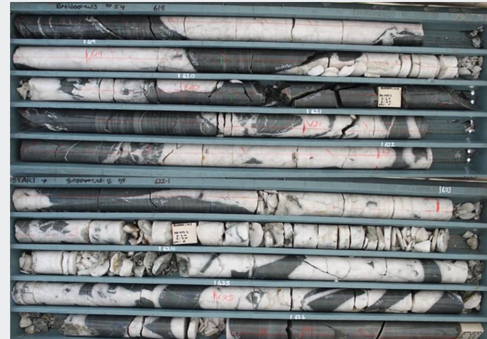
7.6m zone of intense quartz vein development – possible saddle reef in the core of the fold hinge (assays pending)
